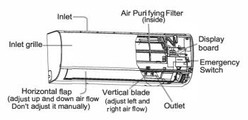
Control the lightening and extinguishing of the indoor LED display board.
