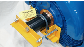
Extensive shaft locking clamp on large AFJE / AFJN motor
