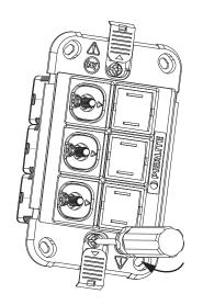
Step 4: Wire the components, then mount the grid plate on the wall. Tighten screws using a Phillips screwdriver.
