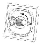
Step 6: Turn the dimmer shaft anti-clockwise until the required minimum brightness level is reached.
