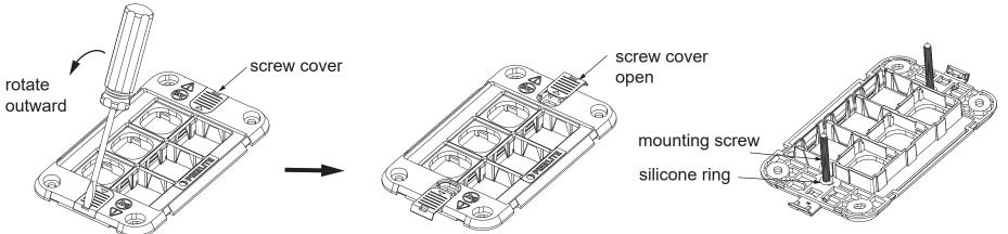
Step 1: Open the screw cover halfway using a flat-head screwdriver.
