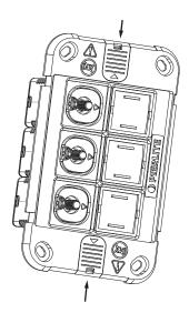
Step 5: Close the screw cover by pushing it with your finger.
