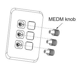
Step 8: Align the triangular maker on the front face of the dimmer with the trianger maker on the inside of the MEDM dimmer knob.
