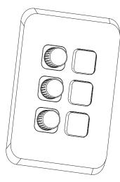
Step 9: Push the dimmer knob onto the shaft so that the triangular markers remain aligned.
