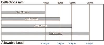
NOTE: The deflections have been provided as a guide based on CONTINUOUS spans.
