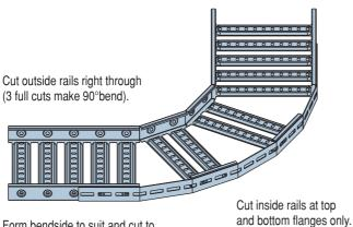
Form bendside to suit and cut to length before fixing to tray with standard joining hardware.
