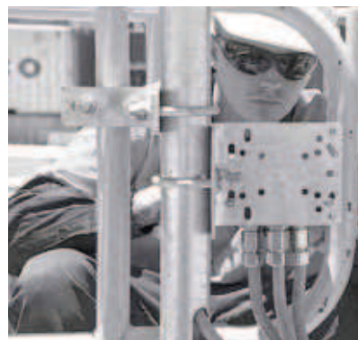
Optional raised junction box plate for easy termination and inspection
