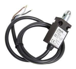
EM14 Series Limit Switch 30mm Aluminium Die Cast Body with 2m pre-wired cable, snap action, Plastic Roller Plunger, 1NO/1NC Contact with double break, 5A/250V AC 0.16A/230V DC switching current, IP67
