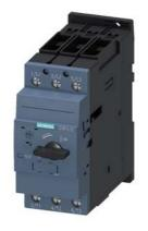
Circuit breaker size S2 for motor protection, CLASS 10 A-release 35...45 A N-release 650 A screw terminal Standard switching capacity
