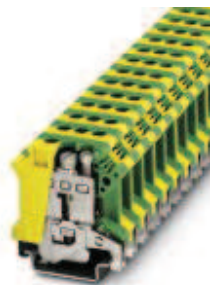
Ground modular terminal block, Screw connection, Cross section: 2.5 mm 2 - 25 mm 2 , AWG: 12 - 3, Width: 12 mm, Color: green-yellow, Mounting type: NS 35/7,5, NS 35/15, NS 32
