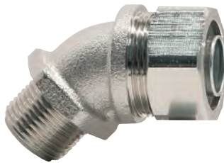
LC - 45 - B (IP66/67/68) External Male Thread 45 degree bend Multi part compression fitting with a nylon seal Available in Zinc Plated Steel, Nickel Plated Brass (B) and 316 Stainless Steel (SS)
