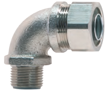
LC-90 - B (IP66/67/68) External Male Thread 90 degree bend Multi part compression fitting with a nylon seal Available in Zinc Plated Steel, Nickel Plated Brass (B) and 316 Stainless Steel (SS)
