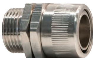
FSC - B - SW (IP40) Two part brass nickel plated straight fitting with a swivel external male thread. Can be installed into a threaded entry or a knockout and secured by a lock nut.
