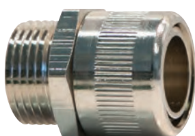
FSC - B (IP40) Two part brass nickel plated straight fitting with a fixed external male thread. Can be installed into a knockout and secured by a lock nut.
