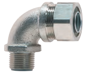
LC-90 - B (IP66/67/68) External Male Thread 90 degree bend Multi part compression fitting with a nylon seal Available in Brass (B) metal and stainless steel (SS)
