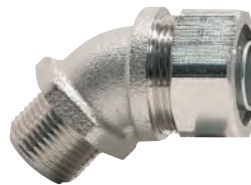
LC - 45 - B (IP66/67/68) External Male Thread 45 degree bend Multi part compression fitting with a nylon seal Available in Brass (B) metal and stainless steel (SS)
