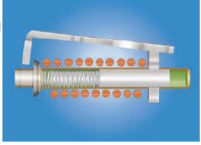
If an overload persists, the core reaches the pole piece with a delay particular to that current. In so doing the reluctance of the magnetic circuit drops so that the armature is attracted to the pole face with sufficient force to collapse the latch mechanism and trip the breaker. The contacts separate, the current stops flowing and the core returns to the reset position.
