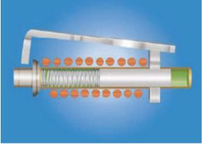
The fluid, creating a time delay inversely proportional to the current dampens the speed of movement. If the overload is of short duration - such as during start up of motors - the core returns to its rest position when the overload disappears.
