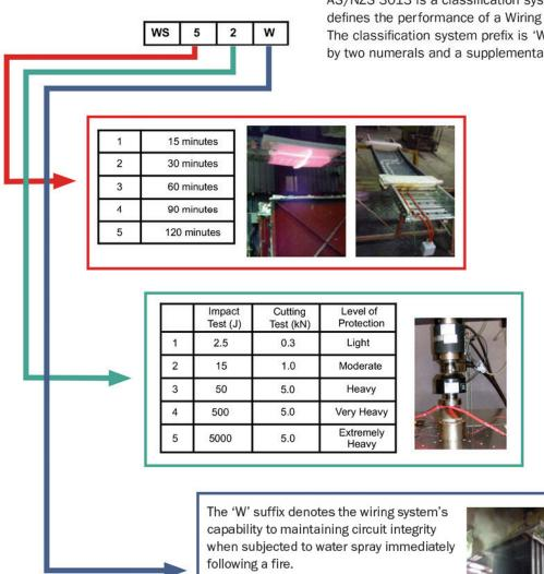
Cables are subjected to fire at 1050°C for 120 minutes, then water sprayed for a further 3 minutes.
