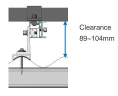
The rail is parallel to the rib of roof
