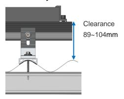
The rail is perpendicular to the rib of roof
