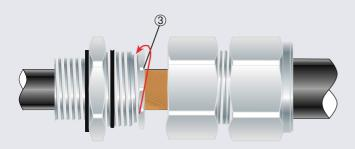
3. Tighten compression nut 3 until coil is in contact with the tape, then turn one full turn.
