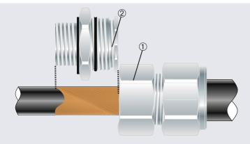
1. Screw outer body ① off and pass cable end through outer body ①. Cut PVC sheath exposing copper tape to the length of inner ②.
