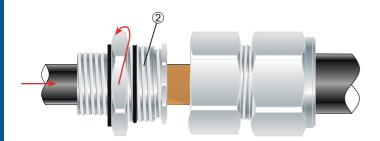
2. Pass cable end through gland inner ② whilst rotating in the same direction as the copper tape.
