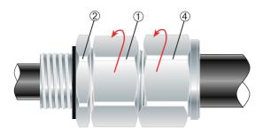
4. Tighten outer body ① over inner ②. Tighten outer compression seal nut ④ .
