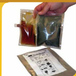
Sealed, two part resin bag
